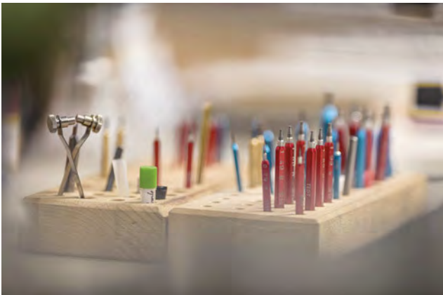
Plug gauges are used to verify the quality of various boreholes
