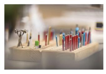
Plug gauges are used to verify the quality of various boreholes
