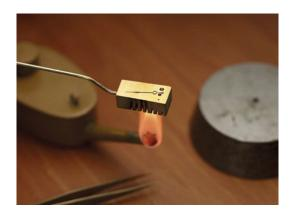
The uniquely sculpted corporeality of the hands is achieved with manual techniques that include grinding with diamond files, edge bevelling, and annealing over an open flame
